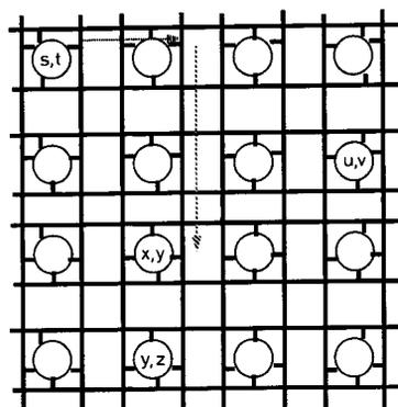
Fig. 4 2-D APW where each processor is connected to four waveguides
